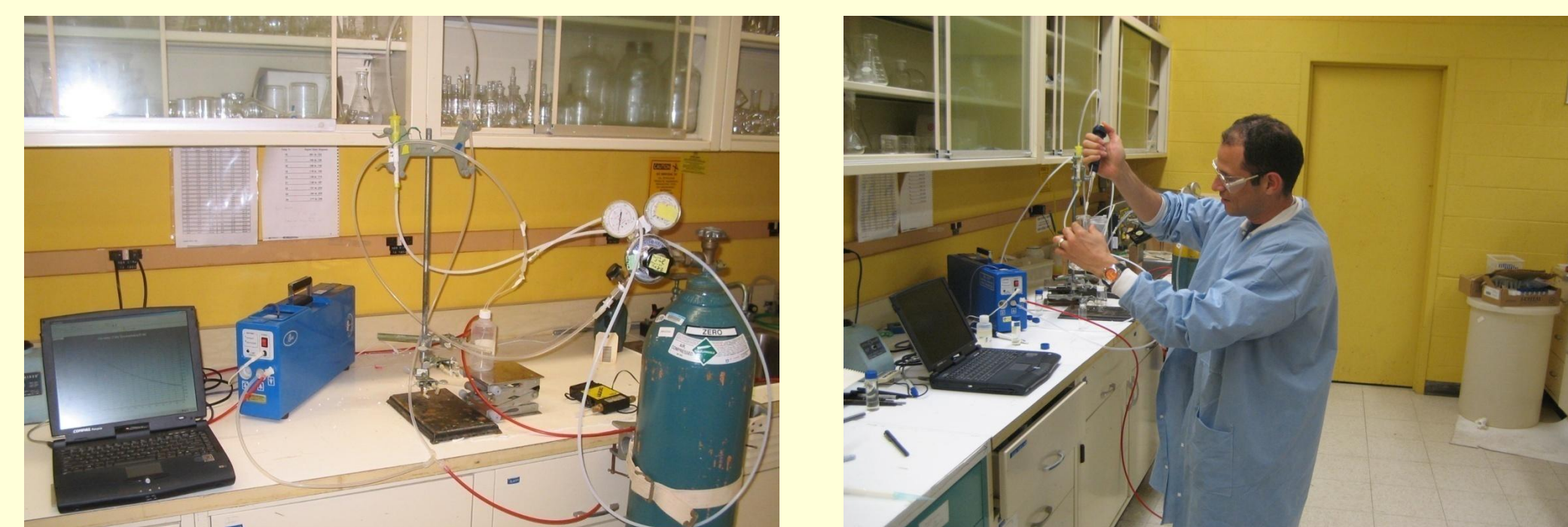
Measurements of Hg(0) concentrations using the Lumex Mercury analyzer and the Mercury Guru software
