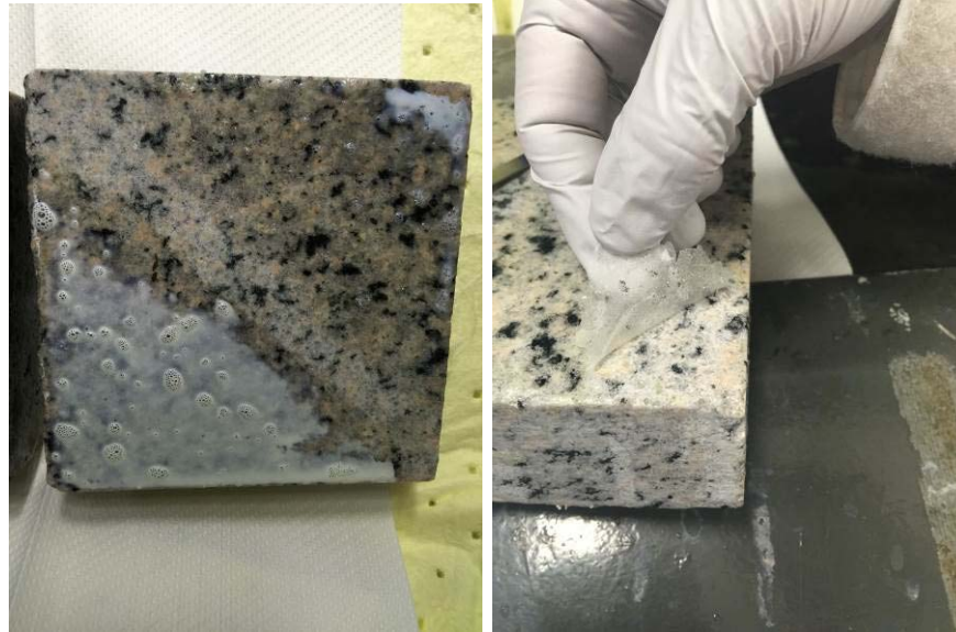
Figure 2. Granite coupon sprayed with solution (left) and pulling off the cured coating (right).
