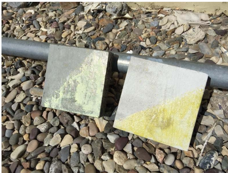
Figure 5. Leached coupon with Product A (left) and non-leached coupon (right).
