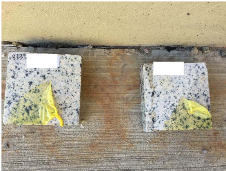
Figure 7. Leached (left) and non-leached (right) coupons cured in the shade (shown once the coating was partially stripped by hand).
