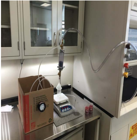
Figure 9. Mock-up scrubber system.
