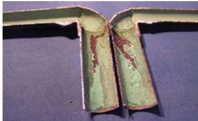
Figure 3. Erosion corrosion within metals.
