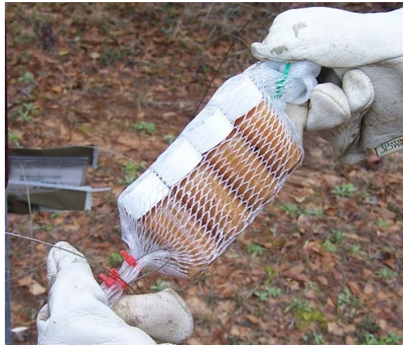
Figure 4: Samplers in plastic mesh.
