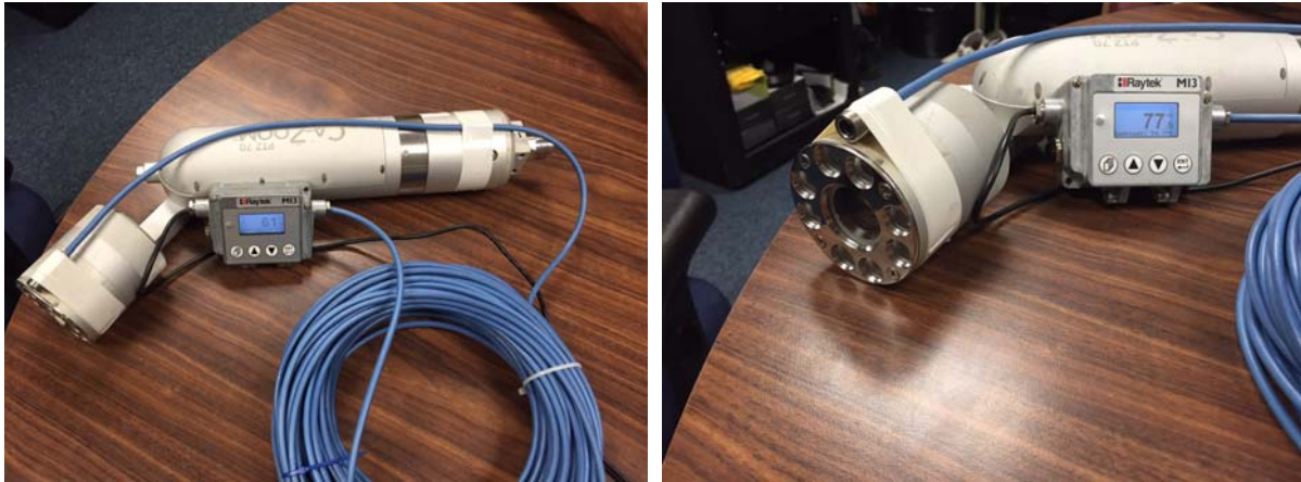
Figure 3. Infrared temperature sensor attached to the annulus inspection camera.
