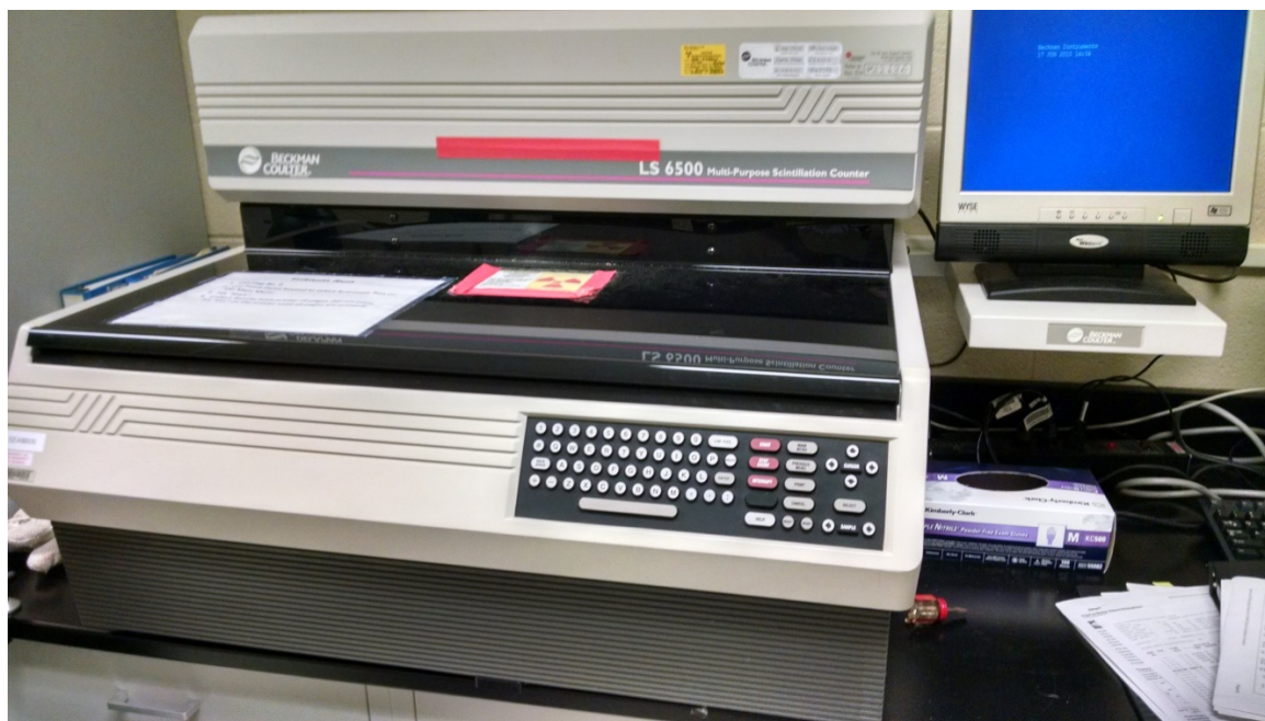
Figure 15. LS 6500 Multi-Purpose Scintillation Counter used in experiment.
