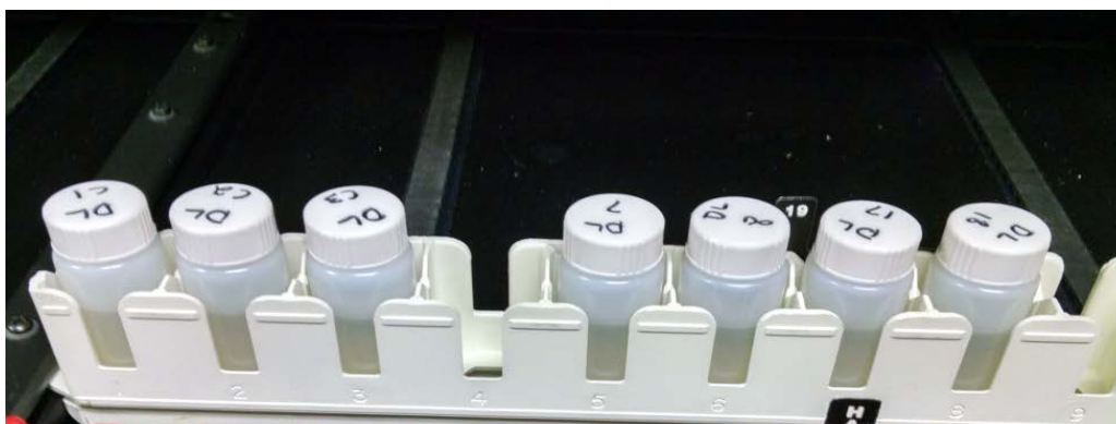
Figure 10. Extracted TWT sample vials loaded onto the Scintillation Counter.
