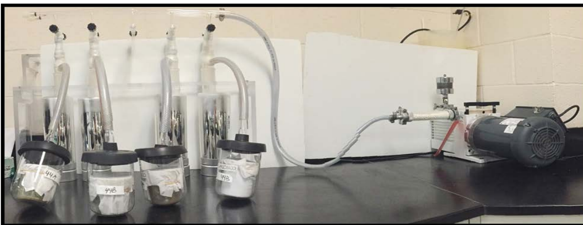
Figure 9. Liquid nitrogen trap used for experiment.
