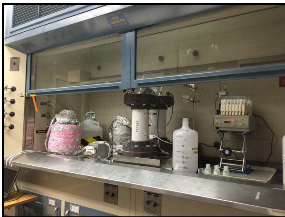
Figure 4. Experimental apparatus constructed in a fume hood. Light sensitive chemicals are contained in foil-covered containers and lines. Pressure sensors monitor for plugging of column and a fraction collector is used to collect samples during final stage of the experiment.
