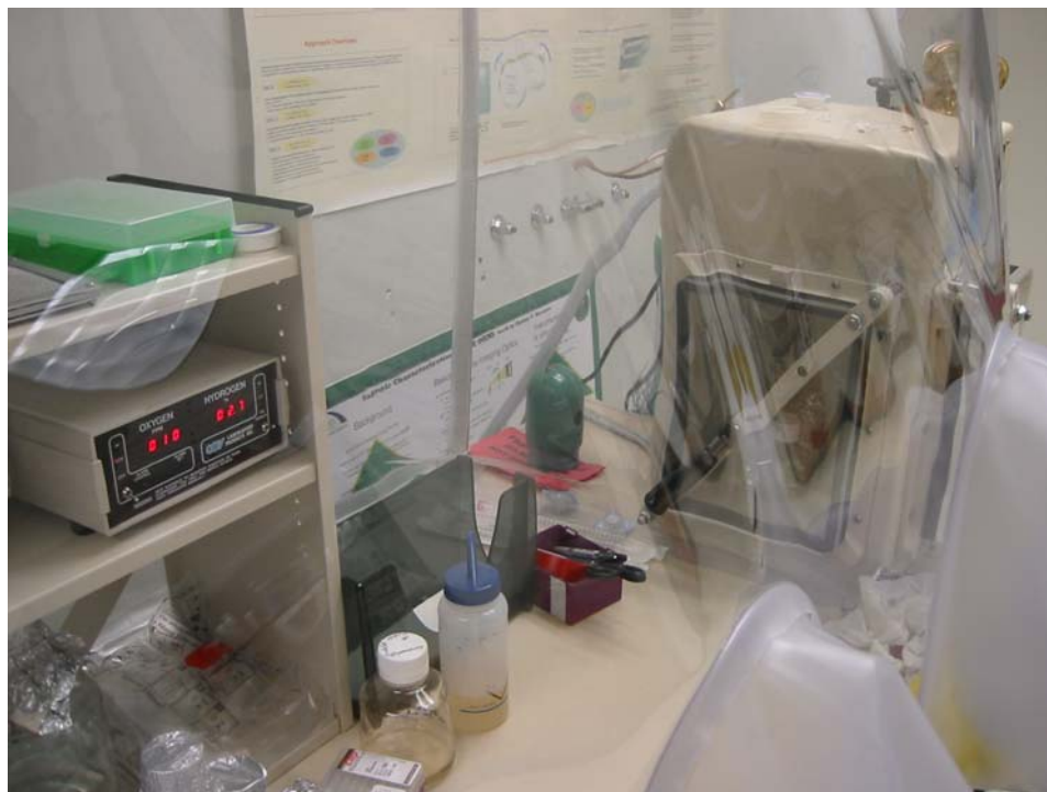
Figure 2: A photograph of an anaerobic glovebag similar to the one used in the experiments.
