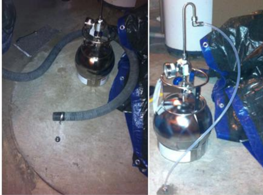
Figure 5. Sub-Slab Sampling at a Residential Site
