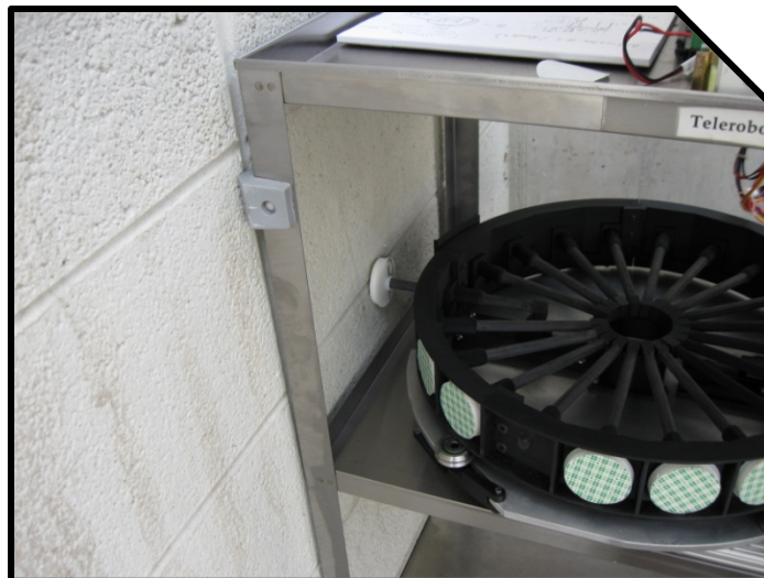
Figure 20: Smear sampler test on semi-rough exterior building wall.
