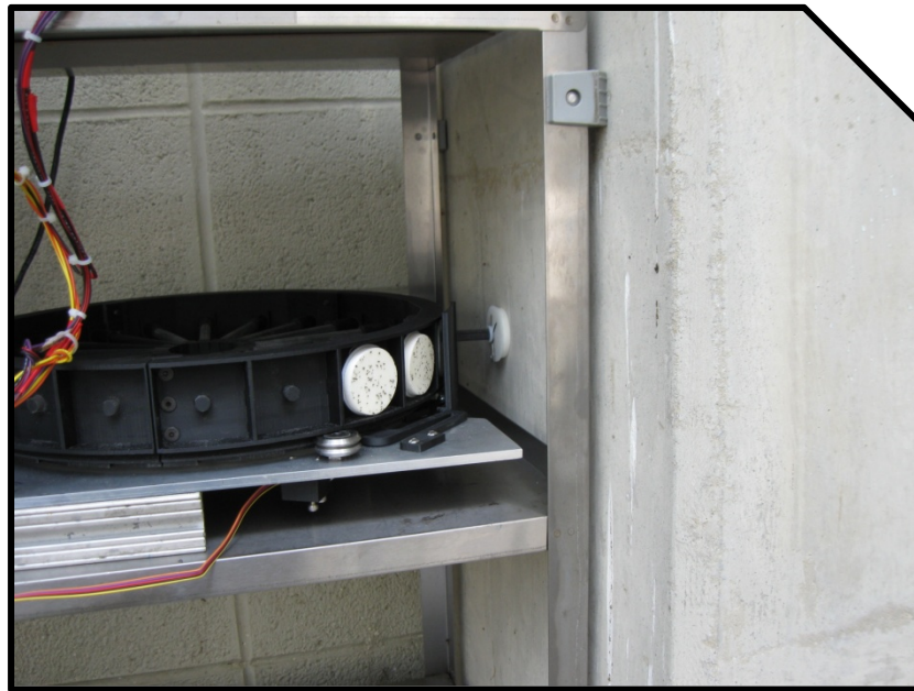
Figure 21: Smear sampler test on smooth exterior building wall.
