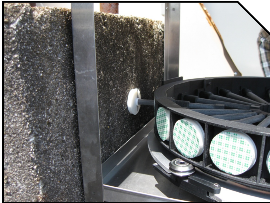
Figure 18: Smear sampler test on concrete block.
