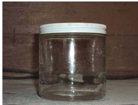
Figure 5: Cellular grout remains floating in water.
