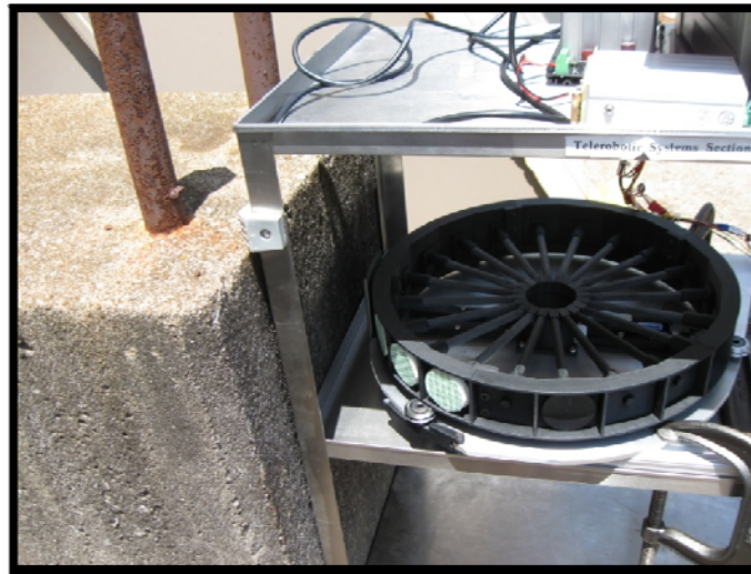
Figure 18. Smear sampler set-up for the experiment.
