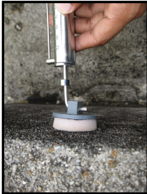
Figure 12. Tension force applied (until retrieval of the pas is achieved).
