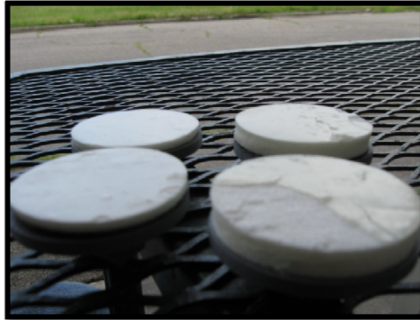
Figure 17. Braking of the adhesive layer of the pad.
