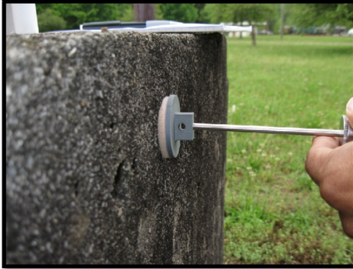
Figure 11. Compression force applied (3 lbf).
