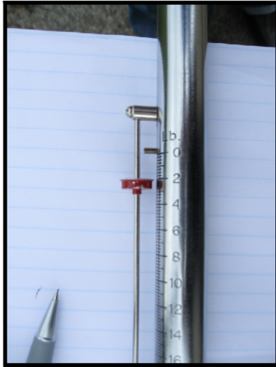
Figure 15. Recording data from spring scale.
