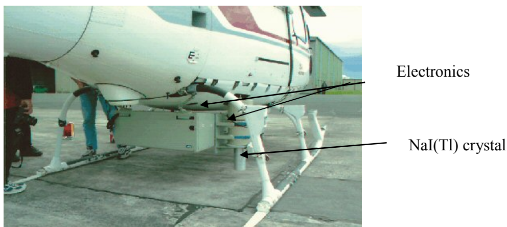
Figure 1. Illustration of detection system in AGRS used for the measurement of radiation from naturally occurring potassium, uranium and thorium in the soils (This experimental setup does not reflect the one used during the NURE program).
