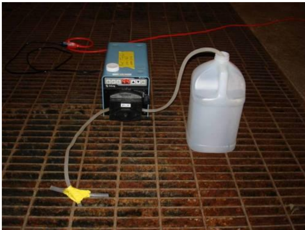
Figure 6. Pumping of Sump I water using a peristaltic pump.
