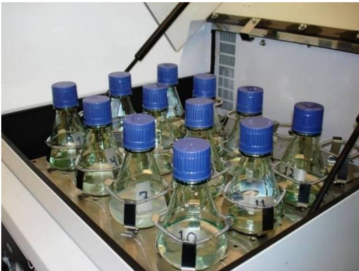
Figure 7. Batch equilibrium tests on a shaker table.
