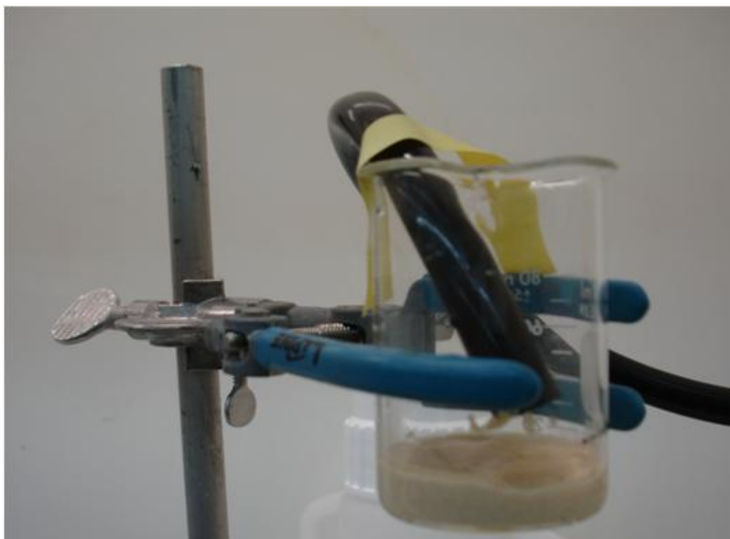
Figure 8. Drying of spent resin.
