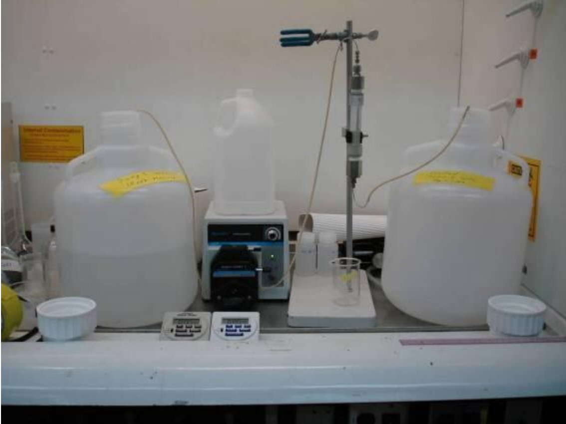
Figure 3. Lab-scale ion-exchange column.
