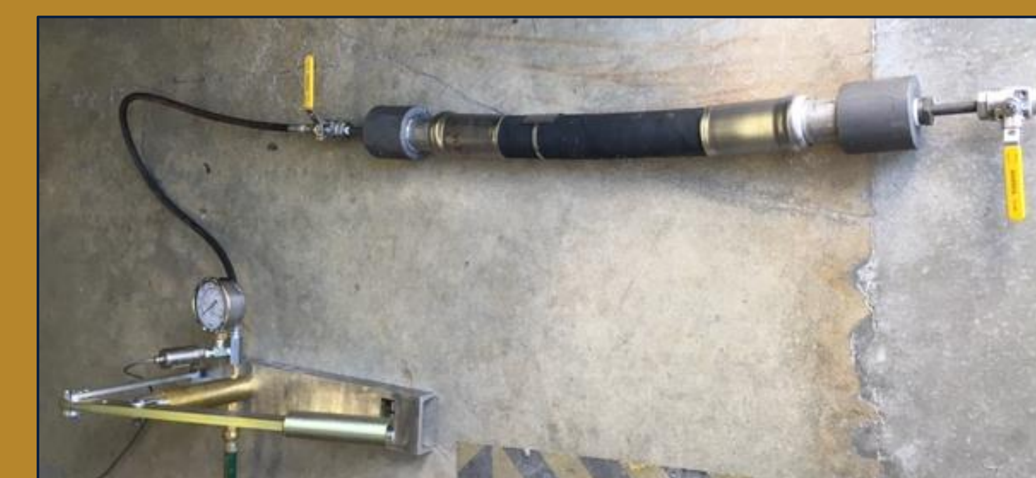
HIHTL Pre-Aging Pressure Test Setup
