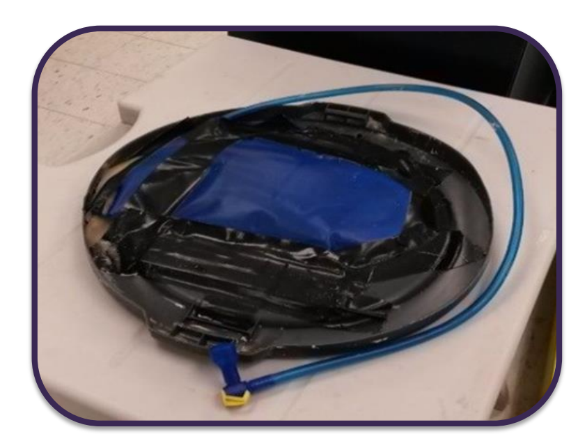
Fig 5: Bladder taped to weighted plastic lid
