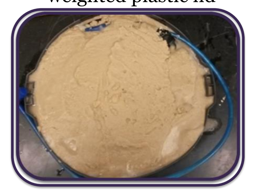
Fig 6: Taped bladder covered with sand
