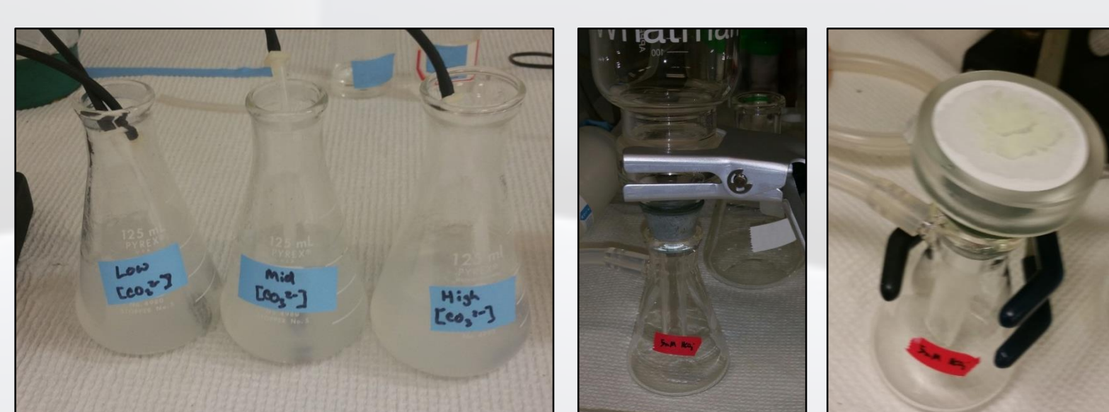
Ammonia gas injection and vacuum filtration steps of the modified sample preparation
