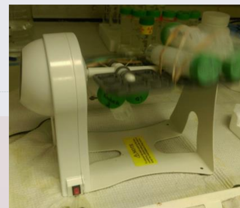
Figure 5. Shaker rotator equilibrating samples at 120 rpm
