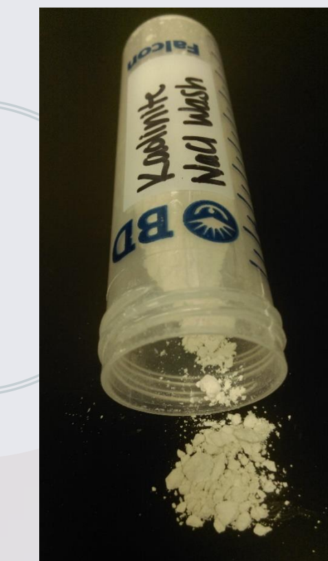
Figure 6. Kaolinite mineral [Al 2 Si 2 O 5 (OH) 4 ]
