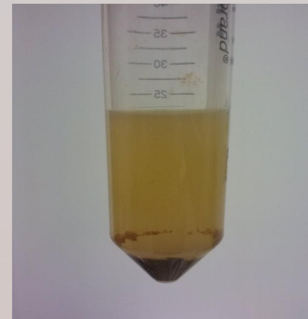
Figure 5. Centrifuge tube with sediment and humate solution
