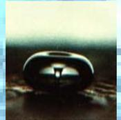
The presence of the solid surface distorts the pressure from the ultrasound field so that a cavity implosion near the surface is asymmetric. This distortion generates a jet of liquid directed at the surface with a speed near 400 km/hr.
