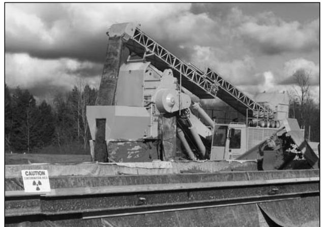
A "one-pass trencher" was used to install a permeable treatment wall to capture Strontium-90 from a groundwater plume.
