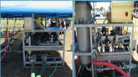
NuVision Engineering pipeline-unplugging skid tested at FIU.
