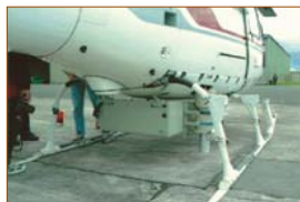
Illustration of a detection system in AGRS (This experimental setup does not necessarily reflect the one used during the NURE program)
