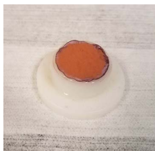
Figure 6. Reactive DGT probe using \text{Cu}(0) reductant without top filter and cap.
