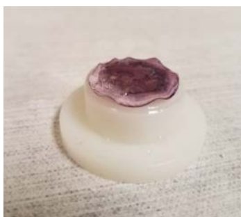
Figure 5. Reactive DGT probe using \text{SnCl}_2 reductant without top filter and cap.
