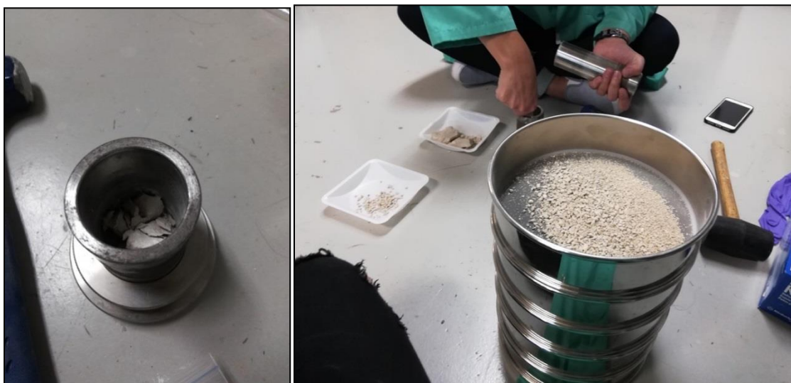
Figure 4. Steel mallet and impact mortar utilized to crush dolomite ( left ) and sieves (No. 45, 100 and 200 sieves) with a variety of different size fractions ( right ).
