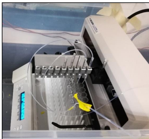
Figure 7: Gilson Fraction Collector (left) and kdScientific 100 Series syringe pump.
