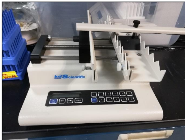
Figure 7: Gilson Fraction Collector (left) and kdScientific 100 Series syringe pump.
