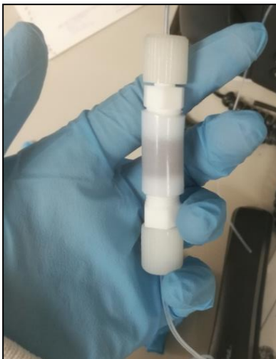
Figure 6. Mini-column setup with fittings attached with inlet and outlet tubings.
