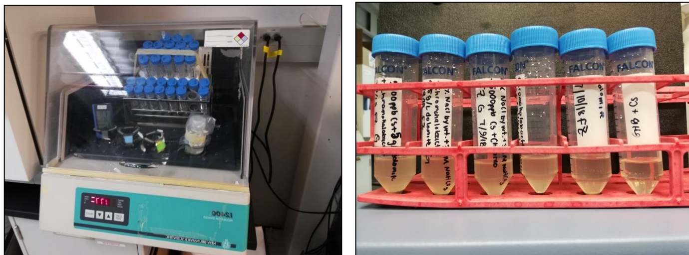
Figure 8. Growth experiment in the incubator shaker (left); the batch samples (right) demonstrate a strong turbidity with the Chromohalobacter over time in terms of growth.
