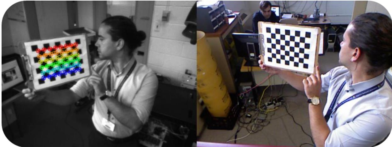
Figure 4. Camera calibration process between left-arm camera and right (head-Kinect) camera.
