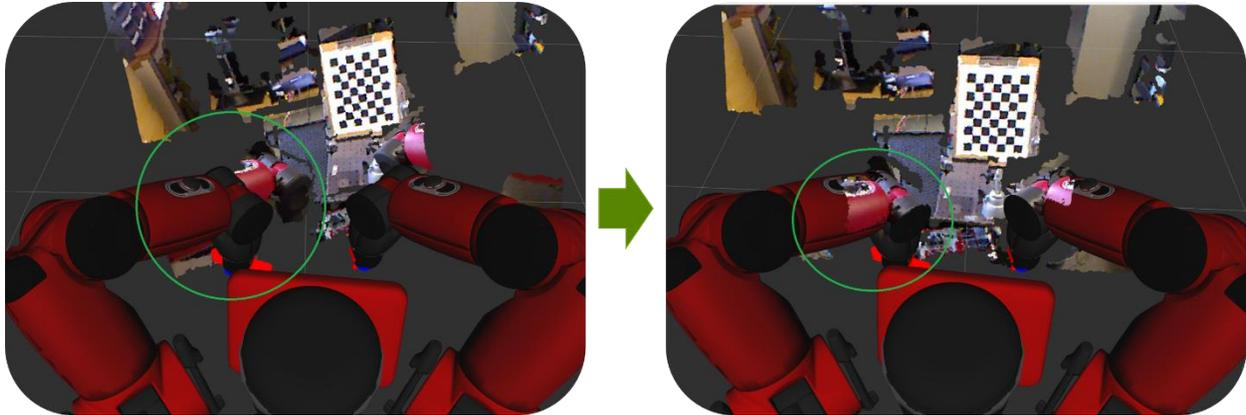
**Figure 6. Before and after camera calibration of Baxter's cameras.**
