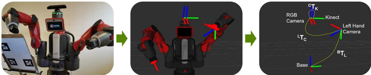
Figure 5. Baxter, Left-hand, and Kinect positions.
