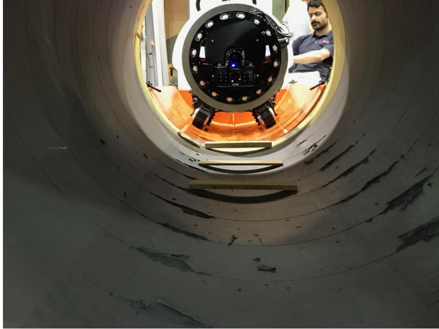
Figure 3. Rectangular modules, located at the bottom of the pipes, being testing.
