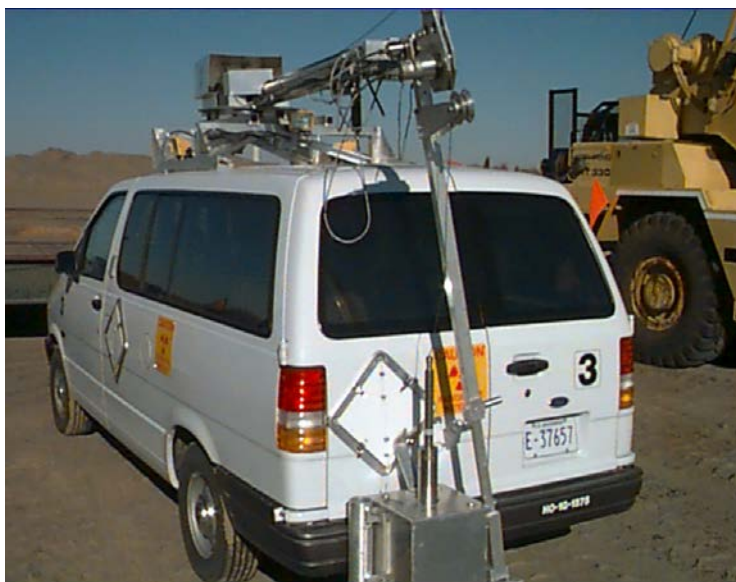
Figure 2. LOW van with ILL attached to gather tank level measurements.
