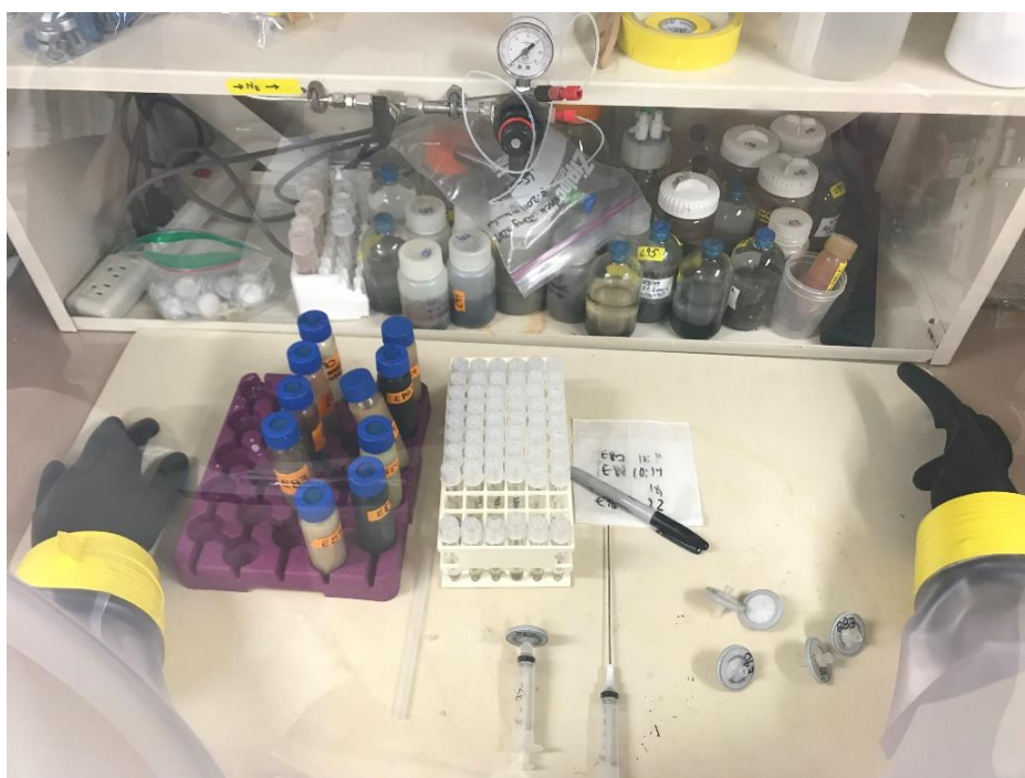
Figure 4. Set-up for sampling day #1 (1 h) of long-term stability of iodine leaching batch experiment.
