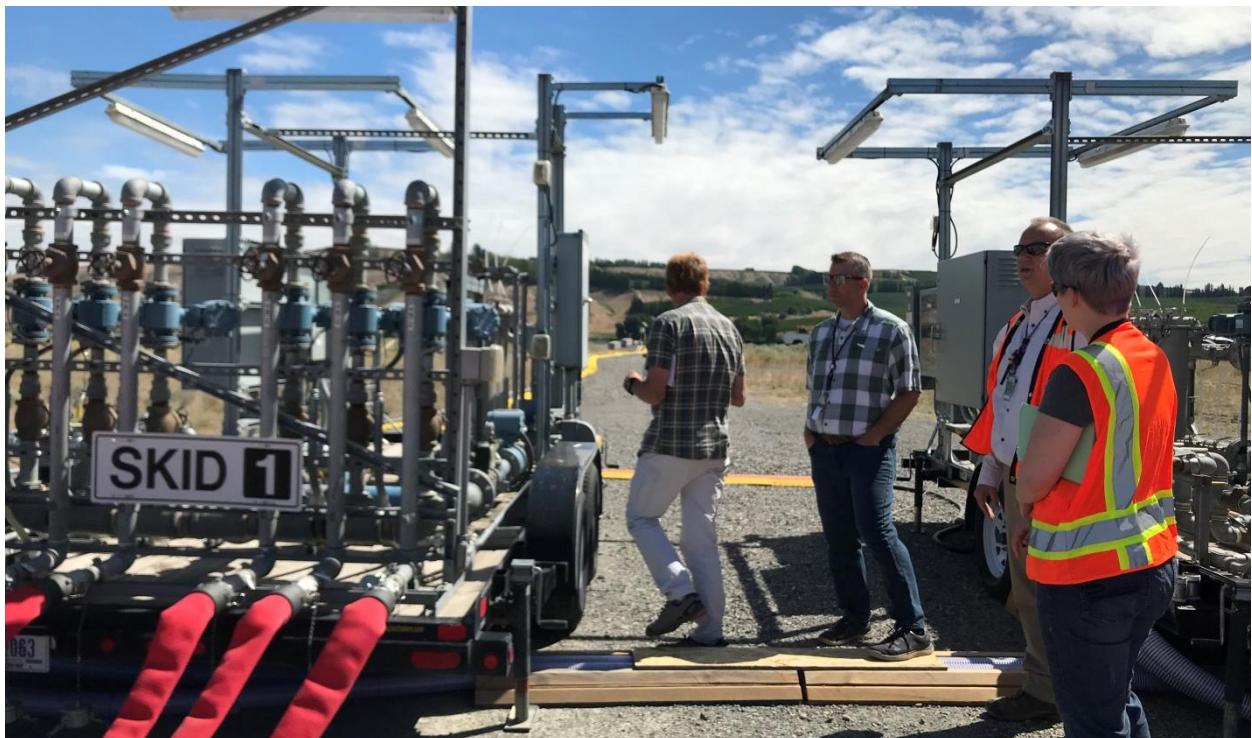
Figure 17. Contractors (right) show PNNL scientists (left) how the pump delivers the polyphosphate solution to the wells.
