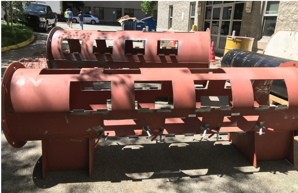
Figure 7. Calibration pipes with sections cut out, to be used for the cold test.
