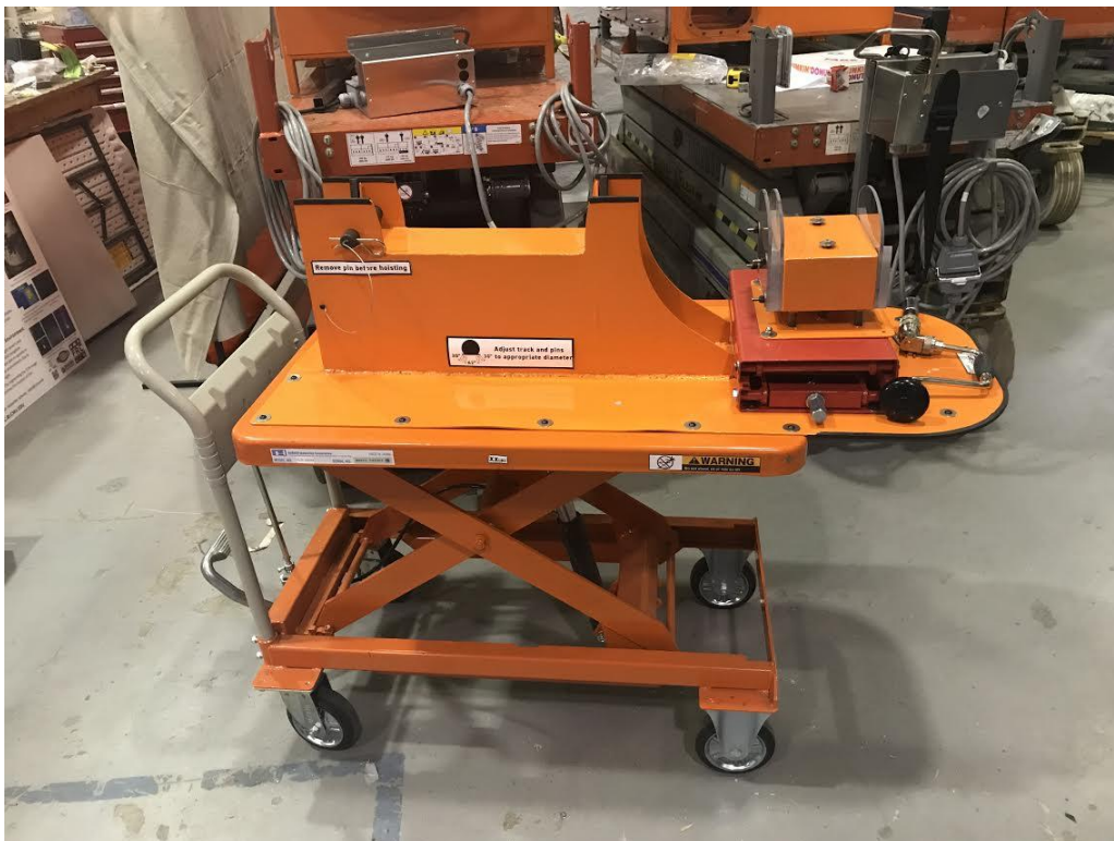
Figure 2. Robot stand that allows for the transformation of RadPiper to either 30” or 42” configuration.
