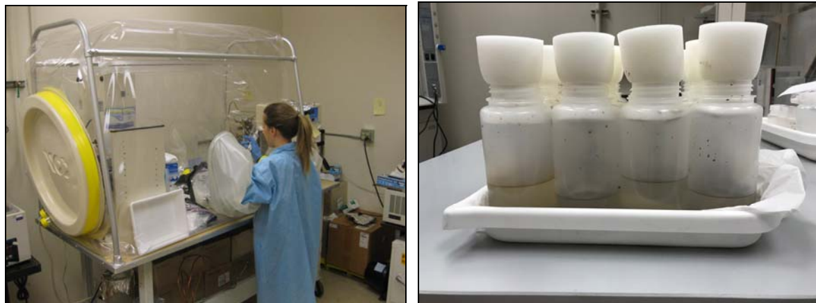
Figure 5: Anoxic batch desorption experiments in glovebox ( left ) and oxic batch desorption experiments ( right ) on the benchtop.
