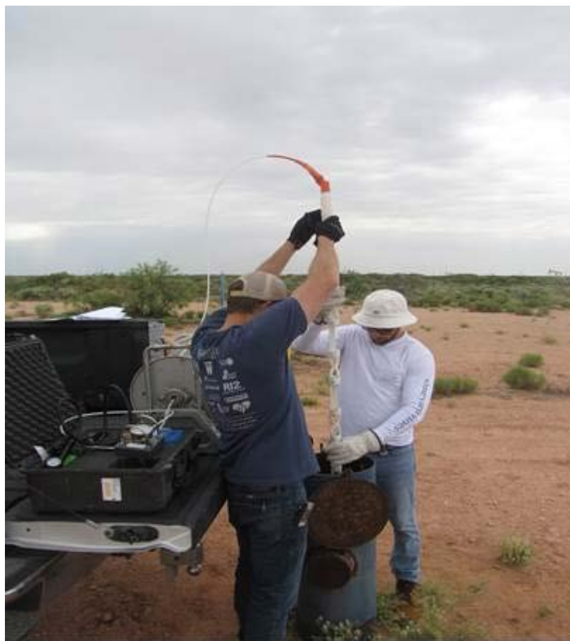
Figure 6: Snap Sampler deployment into well H6-bR using a winch and cable setup of SnapSampler
