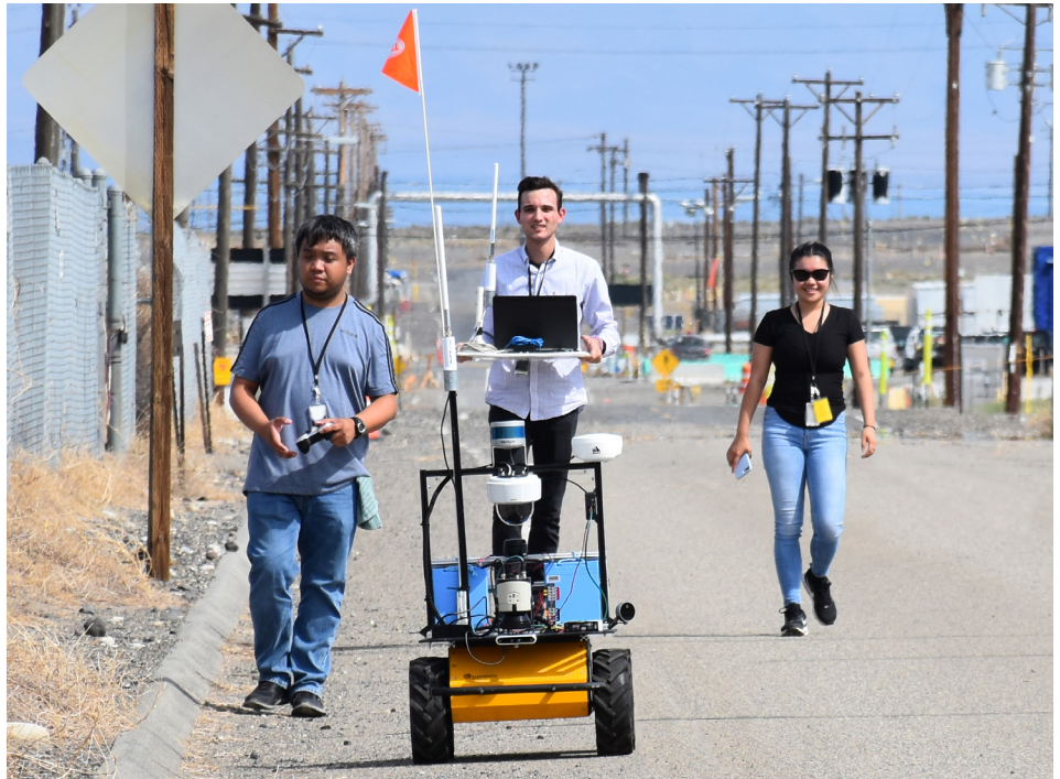
During a recent road closure, Florida International University students (left to right) Jeff Natividad, Joel Adams and Thi Tran test a radiation mapping robot outside of U Farm.
