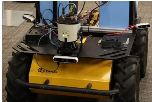
Figure 2. Setup of three depth cameras and onboard computers.
