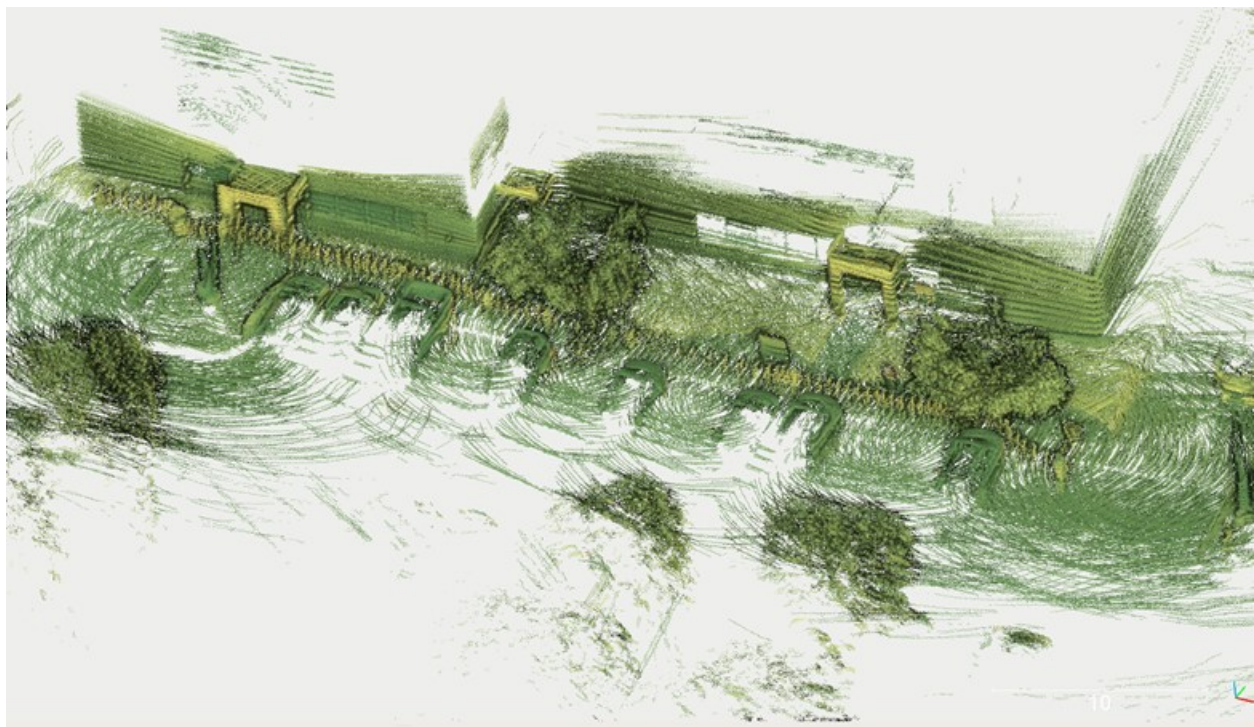
Figure 5. 3D map of north side of building made using Velodyne 3D LiDAR with visual filters applied for enhanced appearance.
