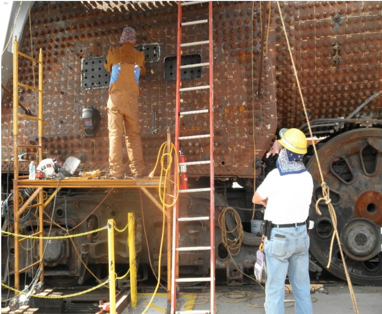
Figure 1. During fire watch, someone must usually be present near the location of the potential hazardous fire, for as long as the hazardous condition exists. Replacing the person with a camera requires introducing forms of machine intelligence to recognize fire in a video stream and generate an alarm.[8]
