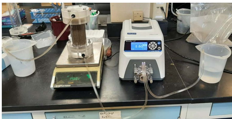
Figure 6. Assembled column test.
