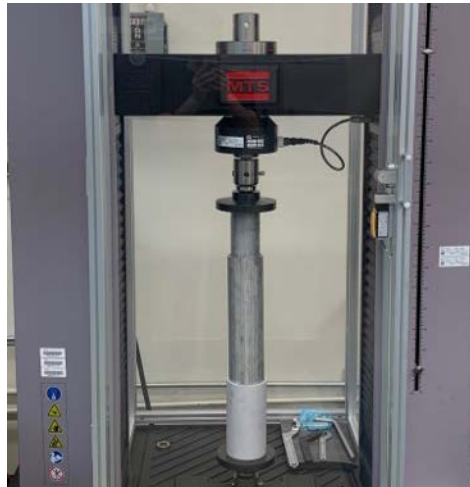
Figure 6. MTS Criterion Tensile Tester Series 43 with aluminum plunger and ABS bucket.
