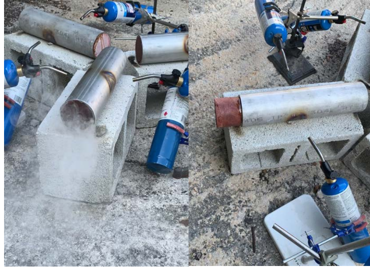
Figure 9. Center-focused flame testing samples producing white smoke (left) and a single sample pushing out a section of Hilti (right).
