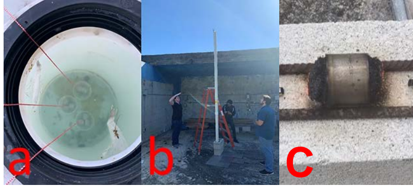
Figure 7. Experimental design of stressors: a) water immersion, b) free drop impact, c) direct flame.
