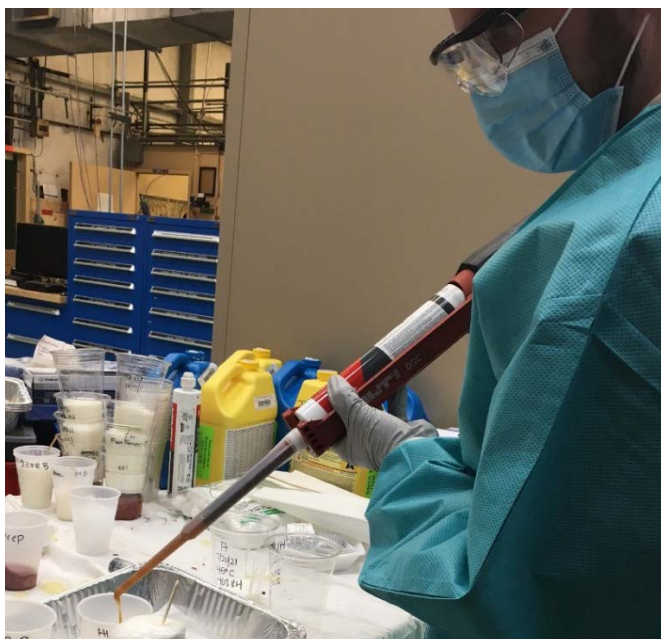
Figure 12. Hilti Firestop foam being applied with the Hilti foam dispenser.
