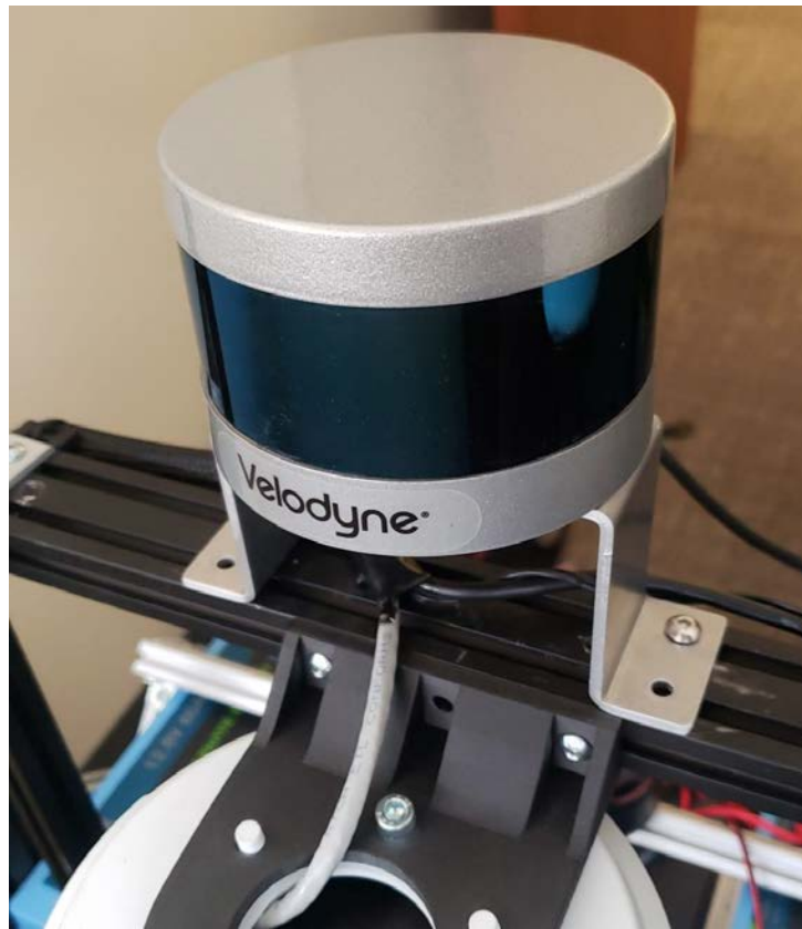
Figure 12: VLP-16 mounted on the Canary.
