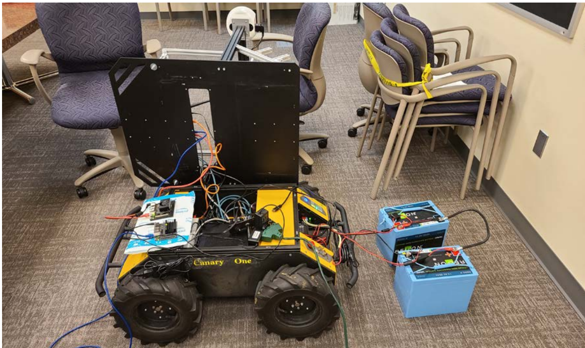
Figure 5: Initial integration of components on Canary without new power system.
