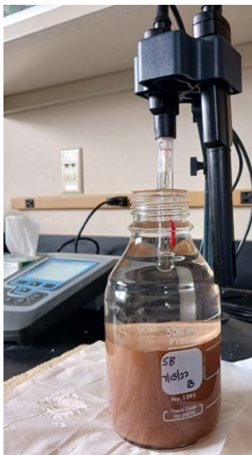
Figure 3. Measuring pH of Sample 5B.
