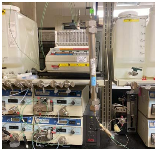
Figure 2: Packed sediment column setup with Hitachi pump and FOXY fraction collector.
