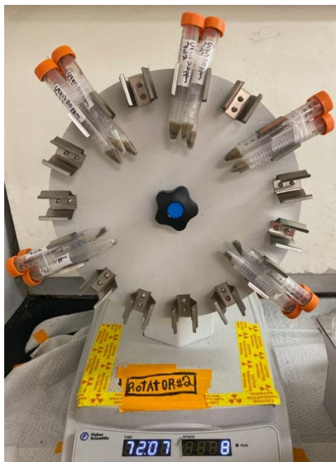
Figure 1: Sediment samples in an end-over-end tube revolver at 8 RPM.
