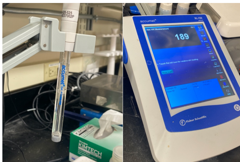
Figure 4: Ion selective probe and meter for Br - analysis.
