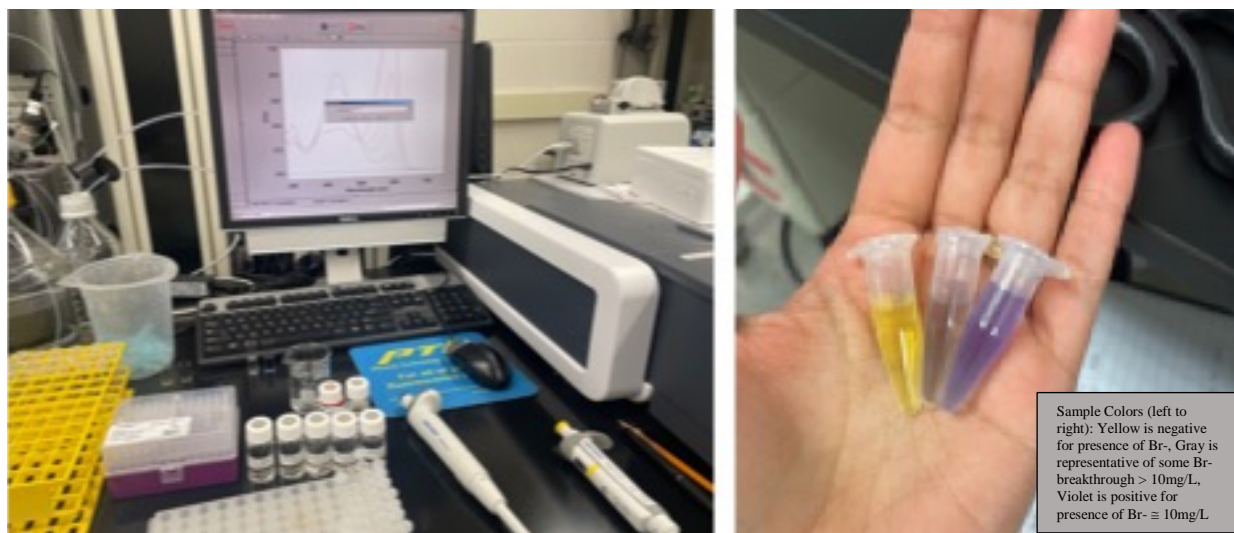
Figure 3 - (left to right) – Agilent Cary UV-Vis Spectrophotometer, Tracer Test Samples Reacted with Colorimetric Assay Reagents
