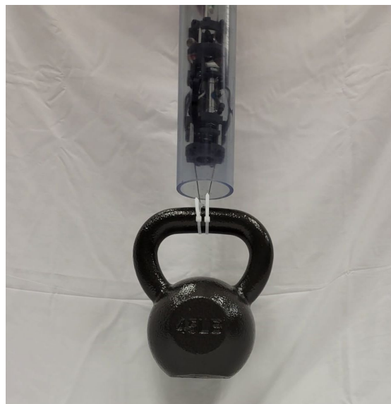
Figure 8. Static Friction Tests for Gripper Module Strength
